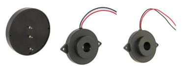
The ABT-466-RC and ABT-467-RC have a feedback option and can be run using either DC or AC voltage. If using a square wave (AC), the feedback pin or lead does not need to be connected. The feedback line on a transducer is used to create a voltage which in turn creates a simple, self-oscillating circuit. A reference circuit is provided on the data sheets. This enables the optimum sound levels to be produced.
